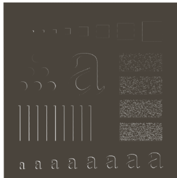
FIGURE 2.37 Image registration. (a) Reference image. (b) Input (geometrically distorted image). Corresponding tie points are shown as small white squares near the corners. (c) Registered image (note the errors in the borders). (d) Difference between (a) and (c), showing more registration errors.
